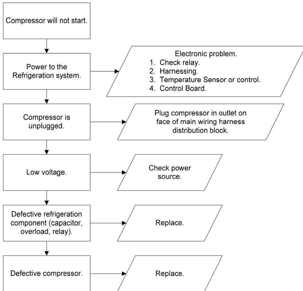
**Troubleshooting Tip:** Use a short 15 Amp extension cord and plug the compressor directly into the wall outlet. This will bypass the Electronic Controls.
