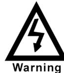
**DO NOT REMOVE THE GROUND PIN ON THE PLUG OR IN ANY WAY BYPASS, MODIFY, DEFEAT, OR DESTROY THE GROUNDING SYSTEM OF THE VENDING MACHINE**
