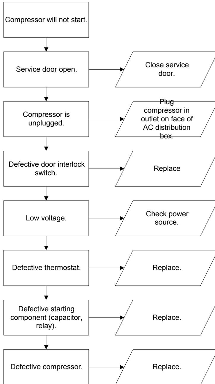
**Troubleshooting Tip:** Use a short 15 Amp extension cord and plug the compressor directly into the wall outlet. This will bypass the AC distribution box.
